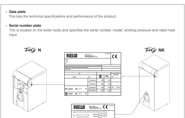
MIf these plates or any other means of clearly identifying the product are defaced, removed or lost, proper installation and servicing may be rendered difficult
