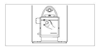
No warning signal is given if the safety thermostat trips, but the fact that is has tripped can be seen from the boiler temperature gauge (T>110°C).
