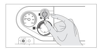
If any ignition faults or malfunctions occur, the burner performs a 'LOCKOUT SHUTDOWN'. This is shown by the red button light on the burner and by the warning light on the control panel.
