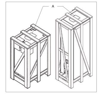
RIELLO TreGi 5/100 ÷ 8/100 NK boilers are delivered in 3 boxes on a single pallet and are further protected by a nylon film.
