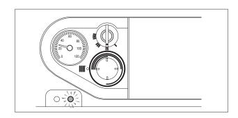
To reset the burner, press the red button light on the burner. The complete ignition cycle will be repeated up to the ignition of the flame.
