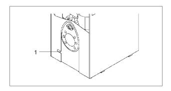
Automatic shut-off device (DAI) (not supplied; only where required).
