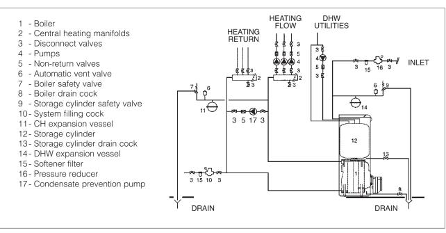
The domestic hot water circuit must include an expansion vessel of adequate capacity as well as a safety valve (max 6 bar), connected directly to the storage cylinder.
