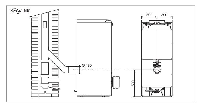
The stack must guarantee the minimum draught specified by applicable technical standards, assuming zero pressure at the connection to the flue gas exhaust.
